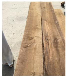
The boards to the right have been fumed for about 4 hours at a high temperature. The effect of fuming and colour changes can be dictated by time as well as heat within the chamber.
