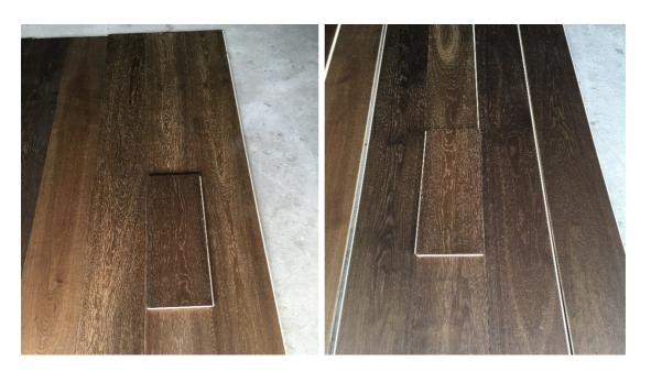
The boards on the right were fumed for 48 hours which means they turned out darker. We then use a colour oil (not stain) to reduce colour variation and finish with 3 coats of UV cured oil to fully seal the surface to create a robust prefinished wood floor.
