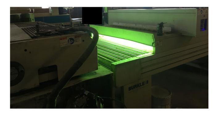
Each station has application rollers that apply accurate measured quantities of the base and top coats. Each of our finishing lines will have 9 application stations as in some circumstance we use the same line for applying our Bona Commercial lacquer system that has 9 coats.
