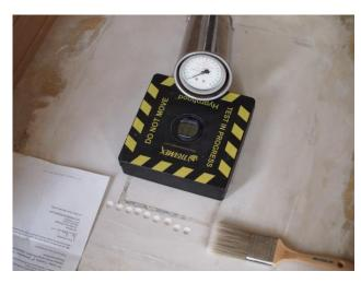
The image on the left shows testing one of these screeds after a vinyl floor (not wood) starter lifting and "bubbling".
