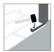
Step 2: Use rubber mallet and pull par to lock short end of plank.
