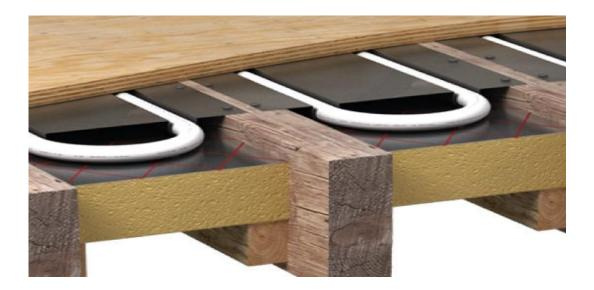
The images below show a slimline underfloor heating system where Impervia can be installed directly on top.
