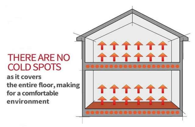
Wood flooring with underfloor heating must be carefully considered as wood reacts to heat and humidity causing it to dry out and contract if the heating is too hot or expand and curl if the humidity is too high. The maximum subfloor temperature for wood flooring is 27 degrees.
