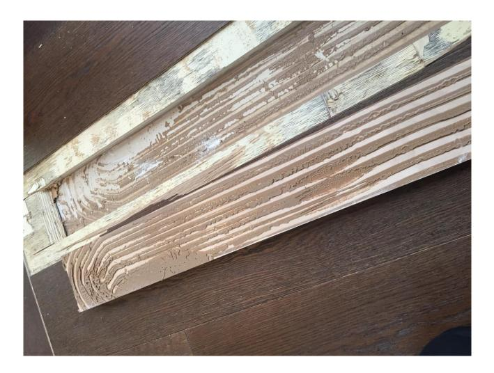
BS 8204 states that you must have a minimum adhesive transference of 75% of the surface area of the plank. In addition, they have used the wrong size trowel and the spacing is to large and not enough adhesive has been applied. Also, the top board in the picture shows large patches of white laitance stuck to the adhesive which means that the laitance have not been removed properly and it is this that has debonded from the screed.
