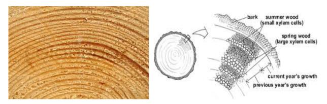
The image below shows the difference between the old heart wood (darker colour) and the younger part which will absorb more moisture and therefore expand and contract more than the middle. As most flooring is now cross cut cupping will occur especially on solid oak wood flooring.
