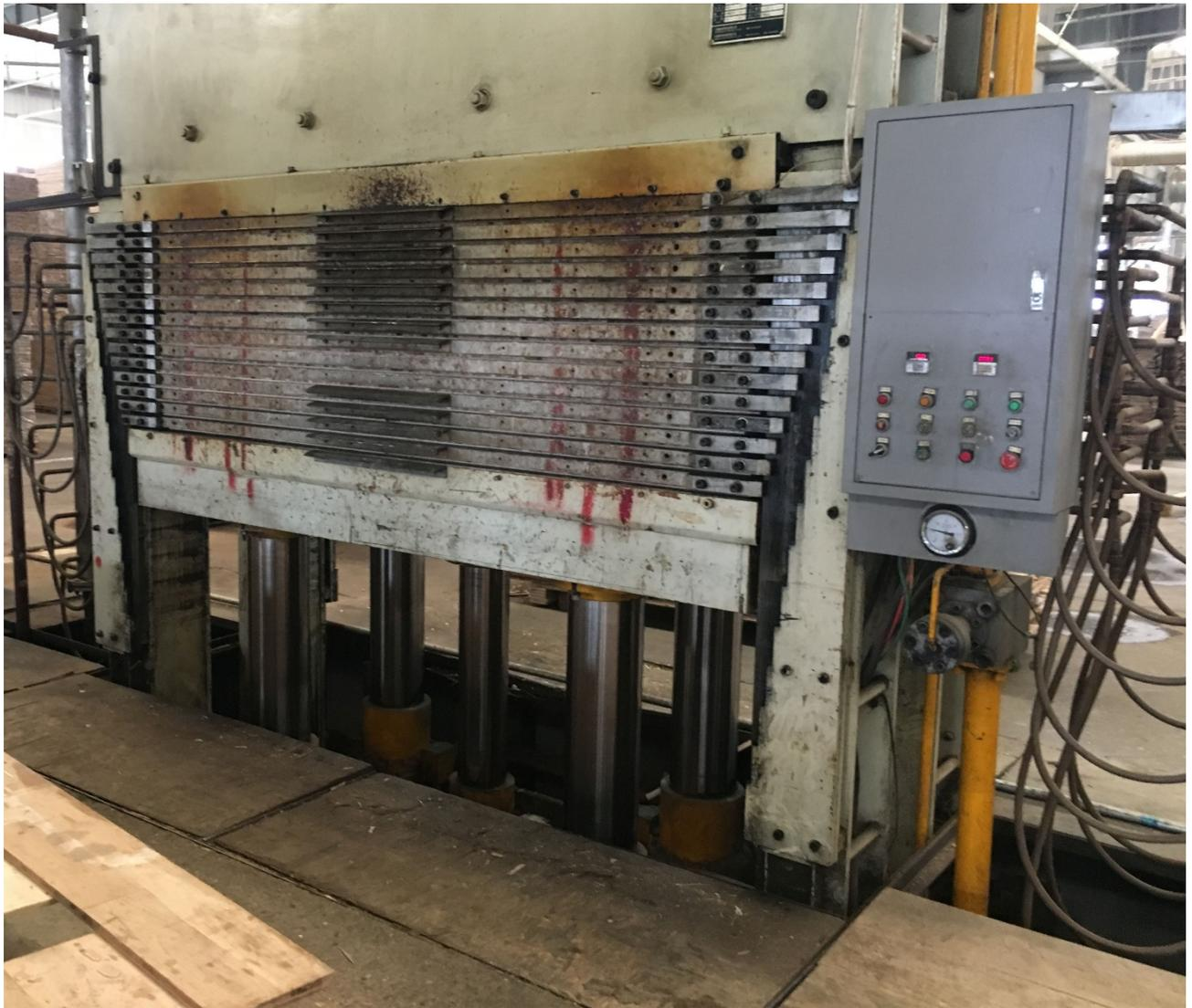
The heat is evenly dispersed through the solid metal plates you can see between each layer. Curing is controlled by the machine and pressure is only released once the adhesive has been fully cured and melted into the cell structure of the wood to create a permanent bond.
