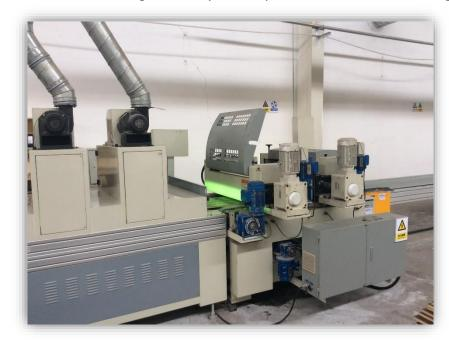
Each station has application rollers that apply accurate measured quantities of the base and top coats. Each of our finishing lines will have nine application stations as in some circumstance we use the same line for applying our Bona Commercial lacquer system that has nine coats. There is also a heating chamber in each finishing line to ensure that the boards are fully dry and in the perfect condition for packing.
